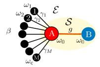
FIG. 1. Schematic of the model: the composite system S is formed of two harmonic oscillators A and B of equal frequency  $\omega_0$  which interact via an exchange Hamiltonian coupling characterized by the constant g. The subsystem A is also coupled with the modes  $k \in \{1, 2, ..., M\}$  of a thermal environment E at temperature  $1/\beta$  (again the interaction is mediated by an exchange Hamiltonian with constants  $\gamma_k$ ).
