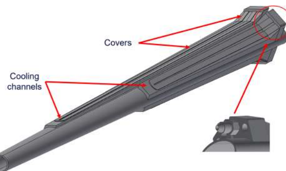
Fig. 83 Left: the central chamber in AlBeMet162 with its cooling inlets and outlets, and its internal gold coating layer. Right: chamber cross section and zoom on the cooling channel for the paraffin flow
