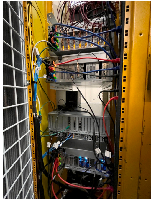
Fig. 4. Photo of the Retina demonstrator in the LHCb Coprocessor TestBed. The server holding the 8 boards is visible at the top, with optic cables running towards the patch panel located above.
