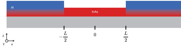
Figure 4.7: Schematic view of the S-N-S junctions. At |x| > L/2 , the InAs nanowire (red region) is partially covered by the Al superconducting leads (dark blue regions). The gray region corresponds to the substrate. This schematic view corresponds to the z - x plane of Fig. 4.3b (top panel).
