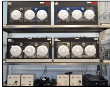
Figure 3.10 Custom-made incubators by Okolab. To replicate clinical conditions for preterm rabbit care, custom neonatal incubators were designed by Okolab (Naples, Italy). Positioned under a walk-in aspiration hood (Weiss Technik, Germany), each incubator consists of a rigid enclosure equipped with oxygen, nitrogen, and temperature sensors, along with a feedback control system to regulate and maintain internal oxygen concentration and temperature.
